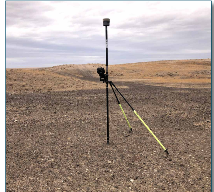
Figure 5: Trimble R10 Model 2 on NVA Survey Point BE007
